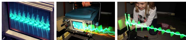
Figure 9. We're often being watched by motion sensors like the microwave sensor of Fig. 2. Left: When we try to look at the received baseband signal from the sensor, as a function of time (artificially spatialized), it is difficult to understand and has little meaning other than a jumble of lines on the screen. Center: When we shut off the timebase of the oscilloscope, and wave it back and forth, we see the very same waveform but displayed naturally as a function of space rather than time. Right: Stephanie, Age 9, builds a robot to move SWIM back-and forth in front of the sensor. As a function of space the displayed overlay is now in perfect alignment with the reality that generated it. This alignment makes physical phenomena like electromagnetic fields more comprehensible and easy to see and understand.
